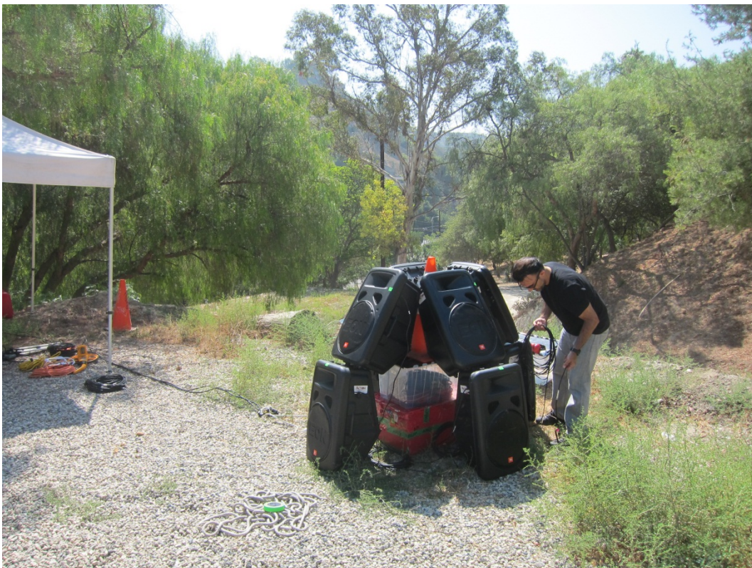
Enlarged view of hemispherical loudspeaker array.
